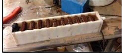
This influent P was chosen because this is similar to P levels found in waterways and agricultural runoff water (0.05 to 0.12 mg/L). As can be seen, P is lowered to below 0.04 mg/L for over 220 days. Readings vary, due to measurement sensitivity in a colorimeter with a limit of ±0.02 mg/L.
